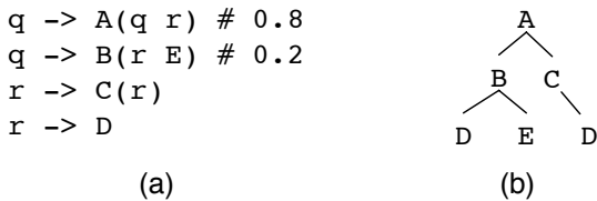
Fig. 2. (a) A regular tree grammar, and (b), a tree in the grammar’s language
